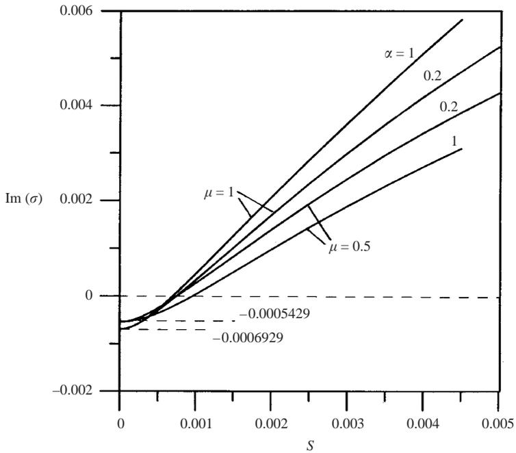
FIGURE 9. Variations of the amplification rate  $\text{Im}(\sigma)$  of streamwise vortices with wavenumber  $\mu = 0.5$  and  $\mu = 1$  induced by the wall transpiration with wavenumber  $\alpha = 0.2$  and  $\alpha = 1$  for  $Re = 5000$  as a function of the transpiration amplitude  $S$ .
