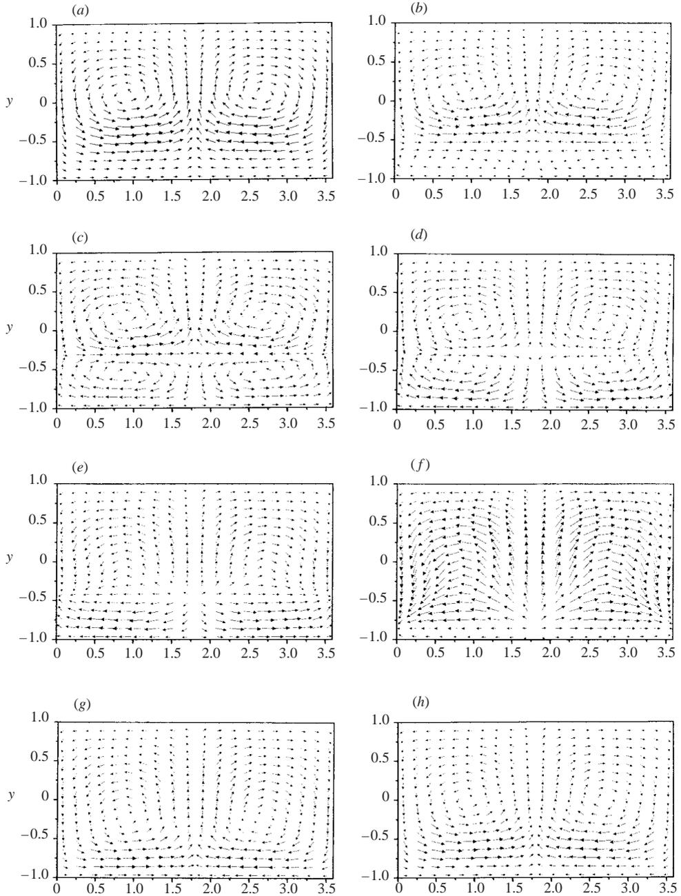
FIGURE 23. Distribution of the  $(y, z)$  component of the disturbance velocity vector for  $z \in (0, 2\pi/\mu)$ ,  $\mu = 1.75$ ,  $\alpha = 1.1$ ,  $Re = 182$ ,  $S = 0.05$ . The disturbance velocity vector is normalized with condition  $\max(g_u^{(0)}) = 1$ . (a–h) Correspond to  $x = 0, \lambda/8, \lambda/4, 3\lambda/8, \lambda/2, 5\lambda/8, 3\lambda/4, 7\lambda/8$ , respectively, where  $\lambda = 2\pi/\alpha$  denotes one wavelength of wall transpiration.
