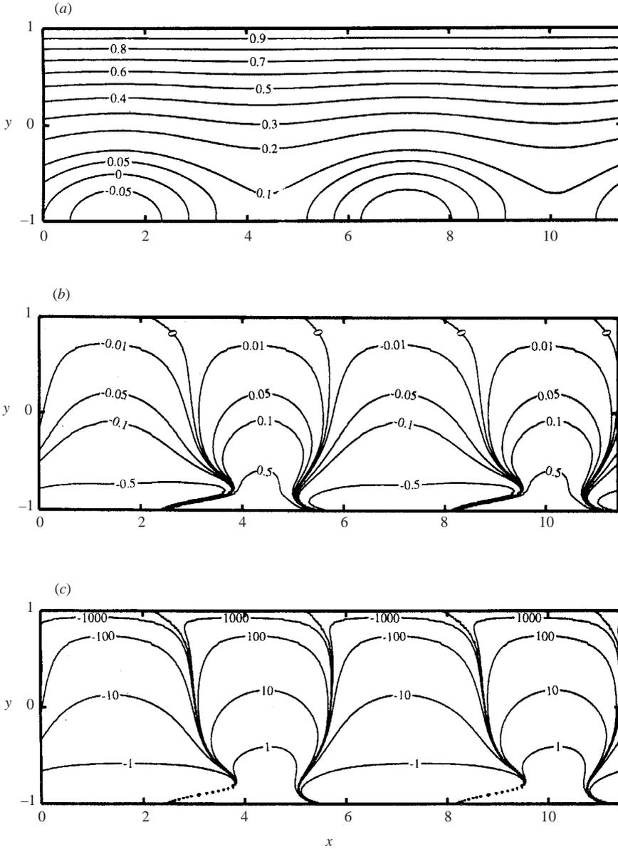
FIGURE 19. Form of base flow resulting from the presence of transpiration with wavenumber  $\alpha = 1.1$  and amplitude  $S = 0.05$  for  $Re = 182$  and  $x \in (0, 4\pi/\alpha)$ . (a-d) Streamline pattern, streamline curvature, (4.1), and circulation, (4.2), respectively.
