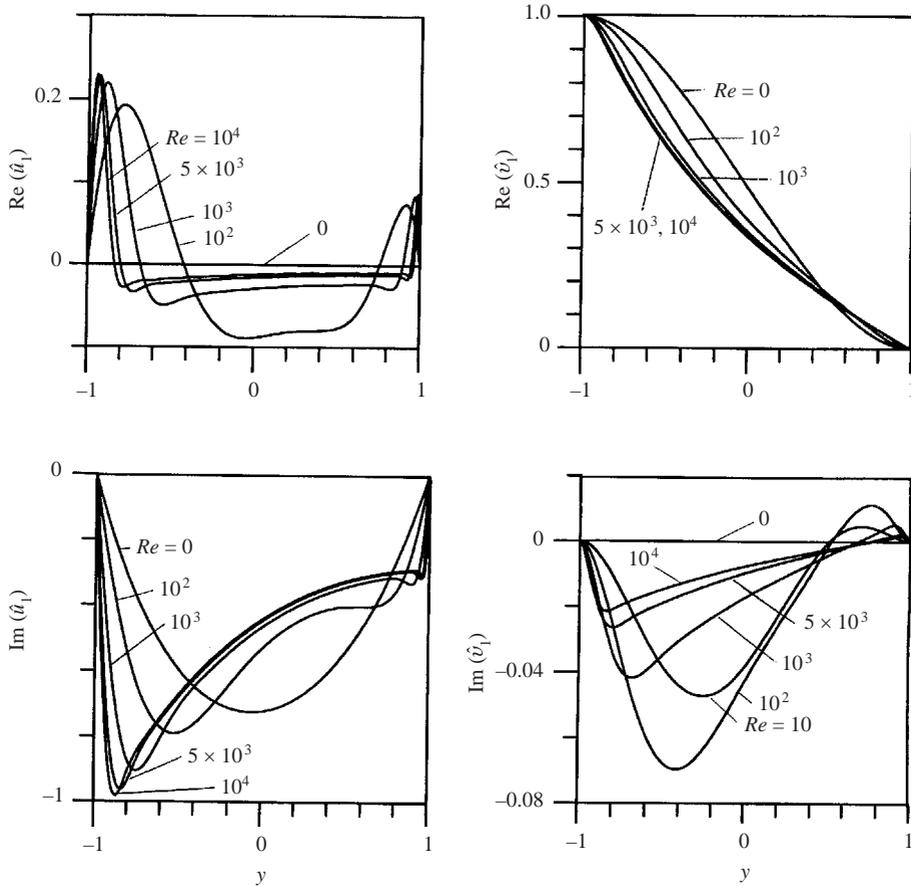
FIGURE 1. Modifications of Couette flow induced by the presence of wall transpiration as a function of the Reynolds number  $Re$  for transpiration wavenumber  $\alpha = 1.0$  obtained with the linear model (§2.4). Hats denote quantities normalized with the amplitude of transpiration  $S$  resulting in  $\hat{v}_1 = 1$  at  $y = -1$ .
