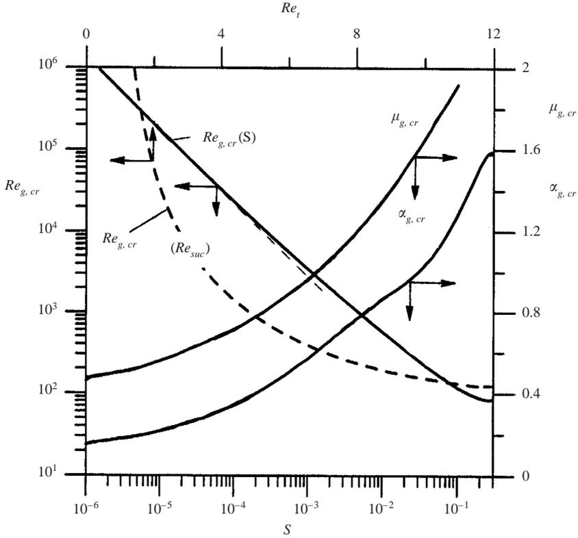
FIGURE 17. Variations of the global critical stability conditions ( $Re_{g,cr}, \alpha_{g,cr}, \mu_{g,cr}$ ) as a function of the amplitude  $S$  of the transpiration. Asymptote for  $Re_{g,cr}$  at large values of  $Re$  is represented with a thin dashed line. Thick dashed line gives variations of  $Re_{g,cr}$  as a function of the transpiration Reynolds number  $Re_t$ . An enlargement of the critical curve for low values of  $Re$  is displayed in figure 18.
