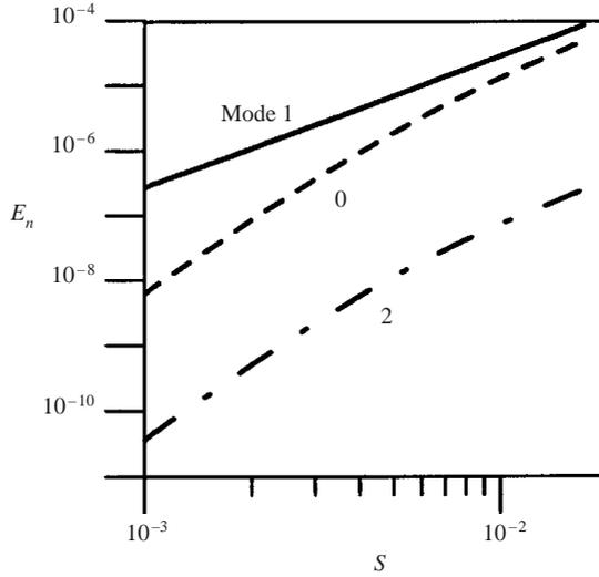
FIGURE 3. Energy  $E_n$  of the first three modes (see (2.11)) associated with the modifications of Couette flow induced by the wall transpiration in the form of a single Fourier mode with wavenumber  $\alpha = 1$  for  $Re = 5000$  as a function of the transpiration amplitude  $S$ .
