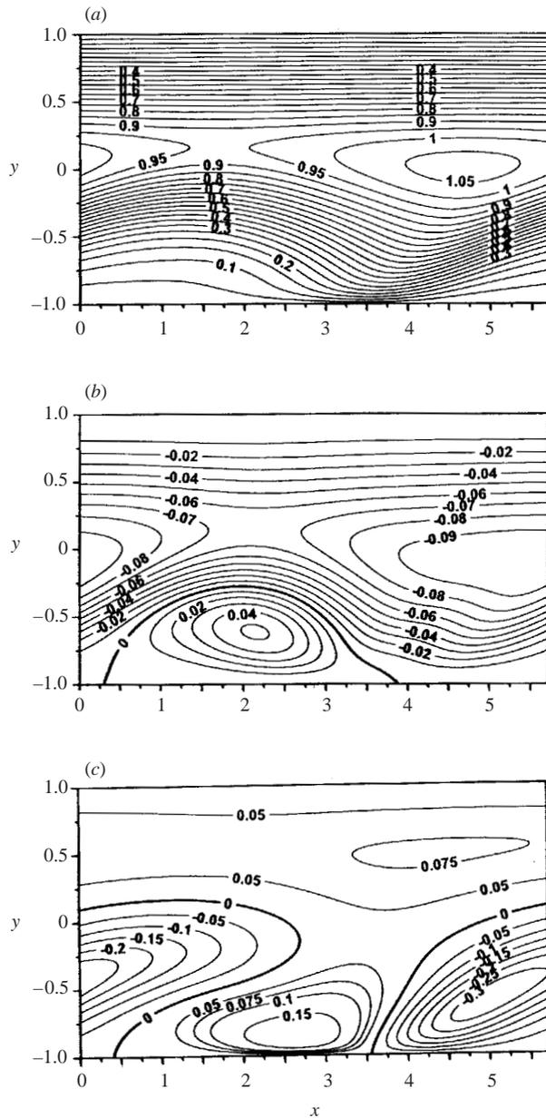
FIGURE 22. Velocity amplitude function  $\mathbf{h}_3(x, y) = [h_u(x, y), h_v(x, y), i\hat{h}_w(x, y)]$  (see (3.5)) for  $Re = 182$ ,  $\alpha = 1.1$ ,  $\mu = 1.75$ ,  $S = 0.05$  normalized with condition  $\max(g_u^{(0)}) = 1$ . (a-c) Functions  $h_u$ ,  $h_v$ ,  $\hat{h}_w$ , respectively.
