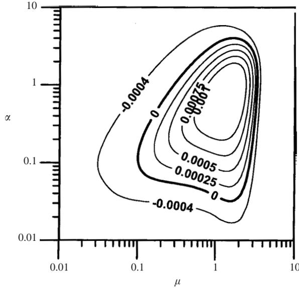
FIGURE 5. Amplification rate  $\text{Im}(\sigma)$  of disturbances in the form of streamwise vortices induced by wall transpiration in the form of a single Fourier mode with amplitude  $S = 0.0015$  for  $Re = 5000$  as a function of the vortex wavenumber  $\mu$  and the transpiration wavenumber  $\alpha$ .
