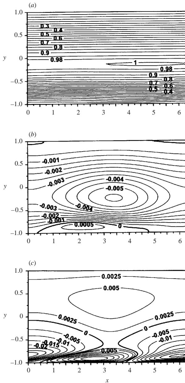
FIGURE 7. Velocity ‘amplitude function’  $h_3(x, y) = [h_u(x, y), h_v(x, y), i\hat{h}_w(x, y)]$  (see (3.5)) for  $Re = 5000, \alpha = 1, \mu = 1, S = 0.0015$  normalized with condition  $\max(g_u^{(0)}) = 1$ . Functions  $h_u, h_v, \hat{h}_w$  are displayed in (a–c), respectively.
