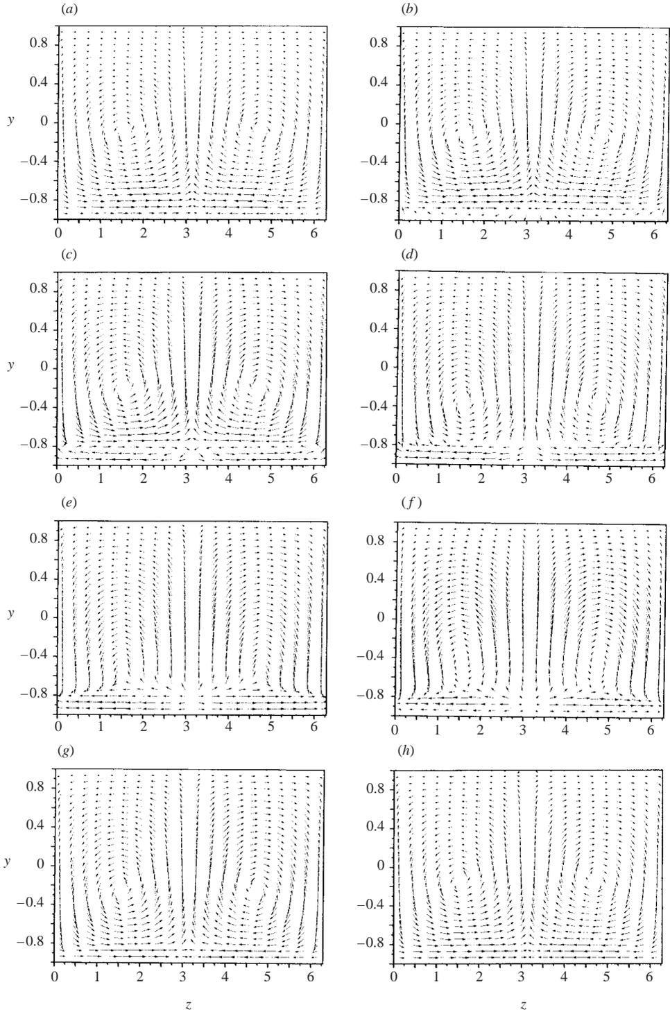
FIGURE 8. Distribution of the  $(y, z)$  component of the disturbance velocity vector for  $z \in (0, 2\pi/\mu)$ ,  $\mu = 1$ ,  $\alpha = 1$ ,  $Re = 5000$ ,  $S = 0.0015$ . The disturbance velocity vector is normalized with condition  $\max(g_u^{(0)}) = 1$ . (a-h) Correspond to  $x = 0, \lambda/8, \lambda/4, 3\lambda/8, \lambda/2, 5\lambda/8, 3\lambda/4, 7\lambda/8$ , respectively, where  $\lambda = 2\pi/\alpha$  denotes one wavelength of wall transpiration.
