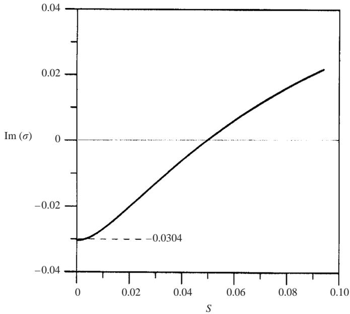
FIGURE 24. Variations of the amplification rate  $\text{Im}(\sigma)$  of streamwise vortices with wavenumber  $\mu = 1.75$  induced by wall transpiration with wavenumber  $\alpha = 1.1$  for  $Re = 182$  as a function of the transpiration amplitude  $S$ .
