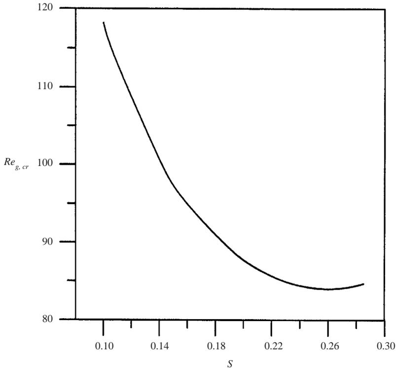
FIGURE 18. Global critical stability curve  $Re_{g,cr}(S)$  for low values of the flow Reynolds number  $Re$ .
