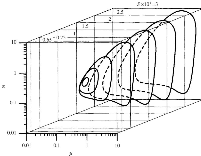
FIGURE 14. The neutral surface describing instability of Couette flow induced by wall transpiration in the form of a single Fourier mode as a function of the transpiration amplitude  $S$ , the transpiration wavenumber  $\alpha$  and the vortex wavenumber  $\mu$  for  $Re = 5000$ .
