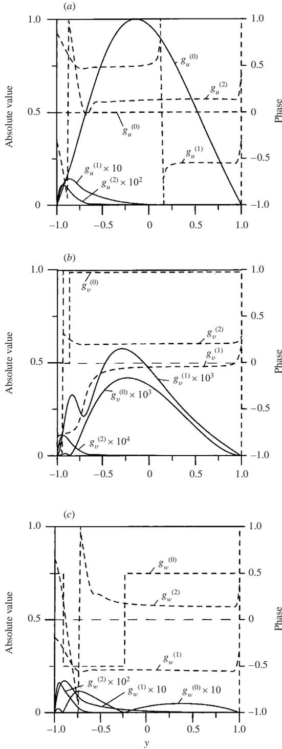
FIGURE 6. Eigenfunctions  $g_u^{(m)}$ ,  $g_v^{(m)}$ ,  $g_w^{(m)}$ ,  $m=0, 1, 2$ , describing a vortex with wavenumber  $\mu=1$  induced by the wall transpiration with wavenumber  $\alpha=1$  and amplitude  $S=0.0015$  for the flow Reynolds number  $Re=5000$  and normalized with condition  $\max(g_u^{(0)})=1$ . (a-c) Functions  $g_u^{(m)}$ ,  $g_v^{(m)}$ ,  $g_w^{(m)}$ , respectively.
