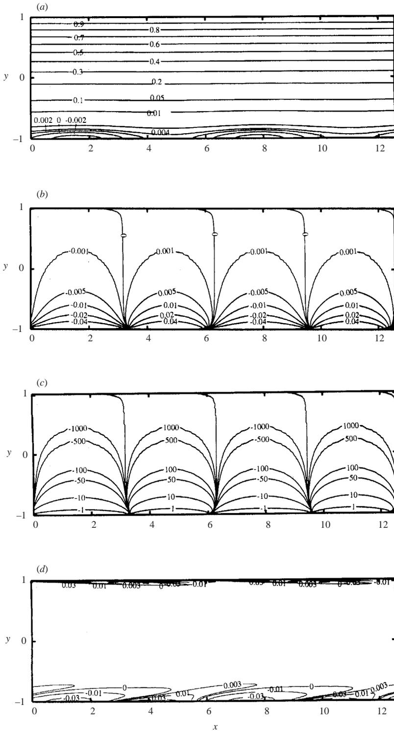
FIGURE 4. Form of base flow resulting from the presence of transpiration with wavenumber  $\alpha = 1$  and amplitude  $S = 0.0015$  for  $Re = 5000$  and  $x \in (0, 4\pi/\alpha)$ : (a-d) display streamline pattern, streamline curvature, circulation and vorticity, respectively.
