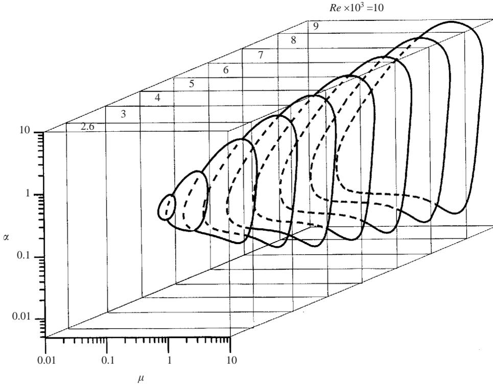
FIGURE 16. The neutral surface describing instability of Couette flow induced by the wall transpiration as a function of the flow Reynolds number  $Re$ , the transpiration wavenumber  $\alpha$  and the vortex wavenumber  $\mu$ . The transpiration has the form of a single Fourier mode with the amplitude  $S = 0.0015$ . The tip of this surface defines the global critical conditions  $(Re_{g,cr}, \alpha_{g,cr}, \mu_{g,cr})$ .
