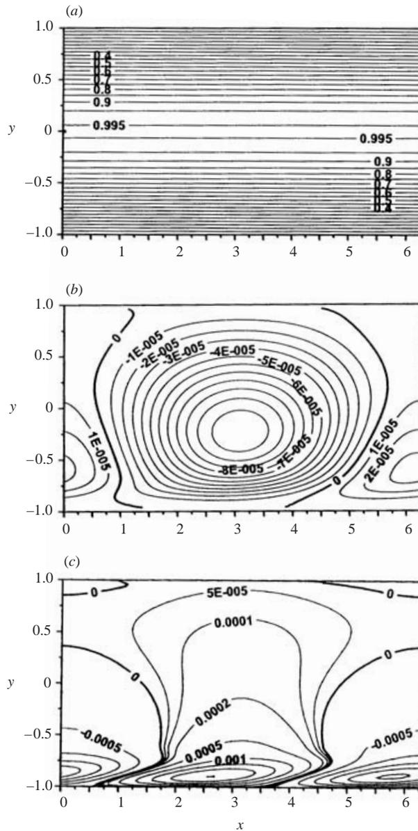
FIGURE 12. Velocity amplitude function  $\mathbf{h}_3(x, y) = [h_u(x, y), h_v(x, y), i\hat{h}_w(x, y)]$  (see (3.5)) for  $S=0.0001$ . The remaining conditions are the same as those used in figure 7. Functions  $h_u, h_v, \hat{h}_w$  are displayed in (a-c), respectively.
