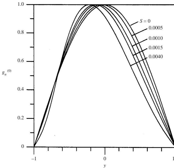
FIGURE 10. Evolution of the real part of the eigenfunction  $g_u^{(0)}$  as a function of the transpiration amplitude  $S$  for  $\alpha = 1, \mu = 1, Re = 5000$ . Normalization condition  $\max(g_u^{(0)}) = 1$ . Since  $g_u^{(0)}$  is real and positive, only  $|g_u^{(0)}|$  is shown.
