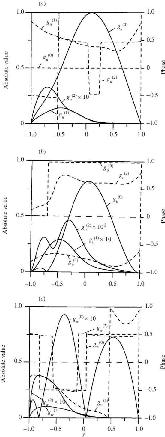
FIGURE 21. Eigenfunctions  $g_u^{(m)}$ ,  $g_v^{(m)}$ ,  $g_w^{(m)}$ ,  $m = 0, 1, 2$ , describing a vortex with wavenumber  $\mu = 1.75$  induced by wall transpiration with wavenumber  $\alpha = 1.1$  and amplitude  $S = 0.05$  for the flow Reynolds number  $Re = 182$  and normalized with condition  $\max(g_u^{(0)}) = 1$ . (a-c) Functions  $g_u^{(m)}$ ,  $g_v^{(m)}$ ,  $g_w^{(m)}$ , respectively.
