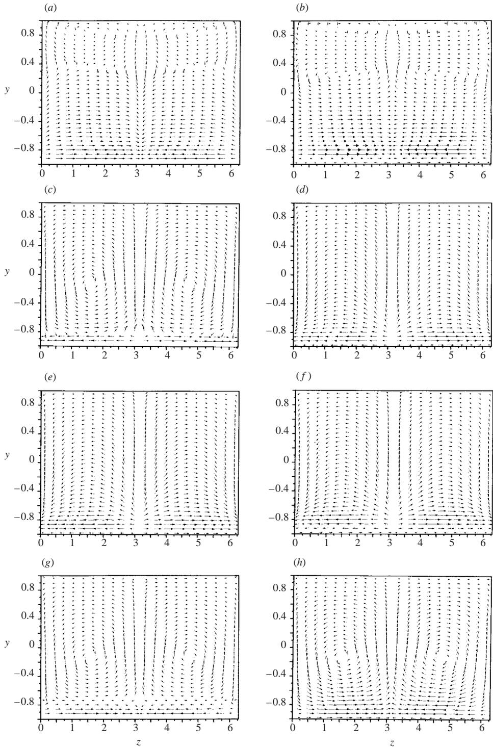
FIGURE 13. Distribution of the  $(y, z)$  component of the disturbance velocity vector for  $S = 0.0001$ . The remaining conditions are the same as those used in figure 8. (a-h) Correspond to  $x = 0, \lambda/8, \lambda/4, 3\lambda/8, \lambda/2, 5\lambda/8, 3\lambda/4, 7\lambda/8$ , respectively, where  $\lambda = 2\pi/\alpha$  denotes one wavelength of wall transpiration.
