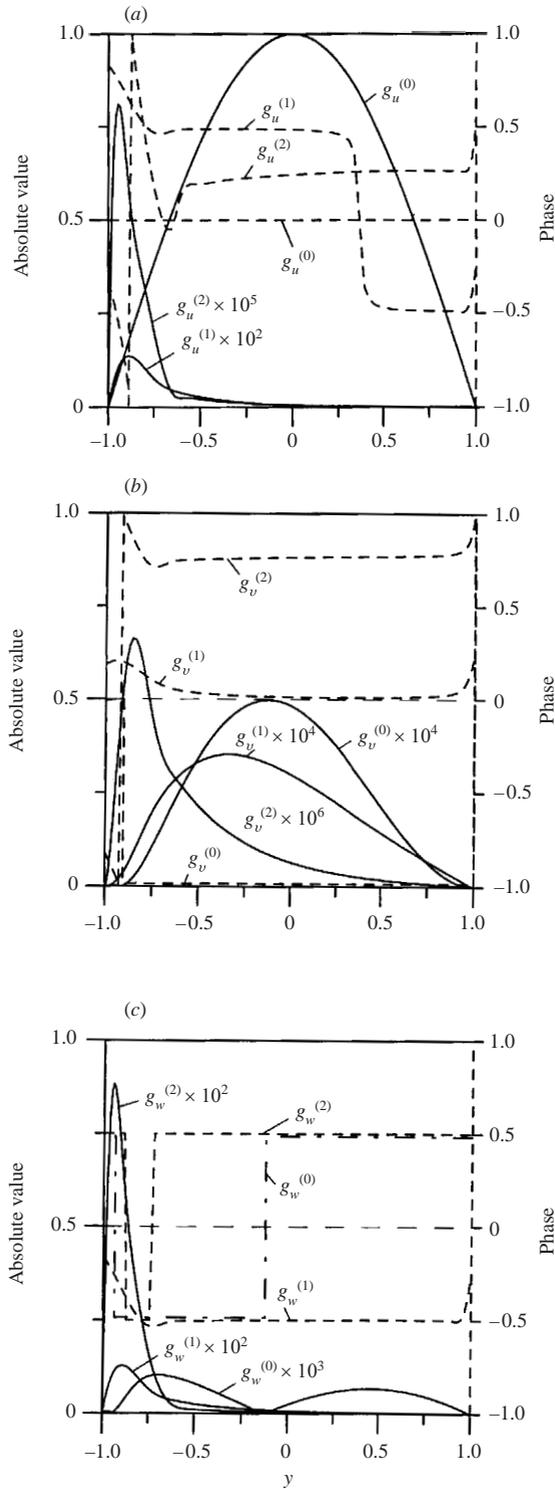
FIGURE 11. Eigenfunctions  $g_u^{(m)}$ ,  $g_v^{(m)}$ ,  $g_w^{(m)}$ ,  $m=0, 1, 2$ , describing a vortex with wavenumber  $\mu = 1$  induced by wall transpiration with amplitude  $S = 0.0001$ . The remaining conditions are the same as those used in figure 6. (a-c) Functions  $g_u^{(m)}$ ,  $g_v^{(m)}$ ,  $g_w^{(m)}$ , respectively.
