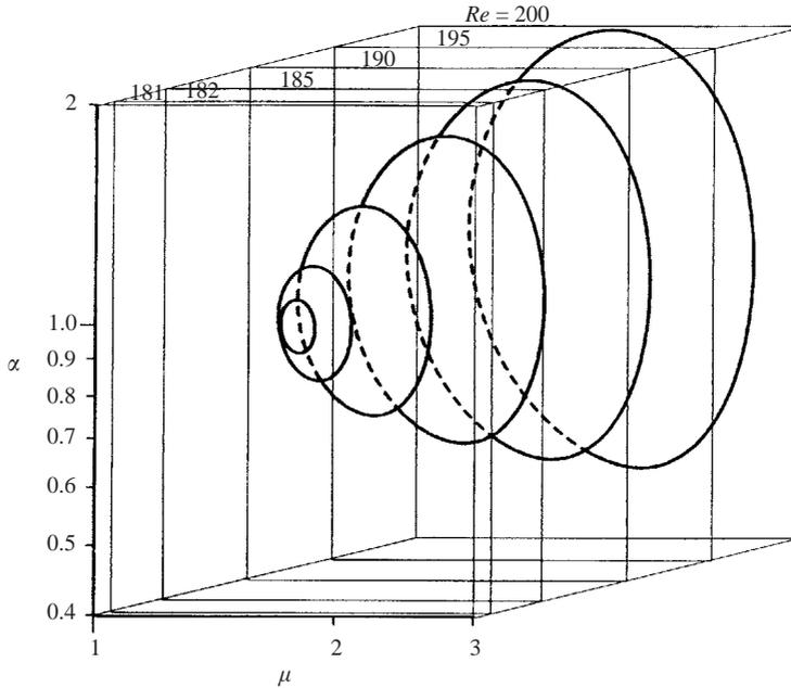
FIGURE 20. The neutral surface describing instability of Couette flow induced by wall transpiration as a function of the flow Reynolds number  $Re$ , the transpiration wavenumber  $\alpha$  and the vortex wavenumber  $\mu$ . The transpiration has the form of a single Fourier mode with the amplitude  $S = 0.05$ .
